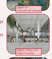
High ceilings and ventilation openings at the top allow warm air to rise and exit.
